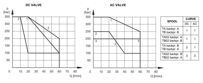
Operating limits of a 4-way valve in 3-way operation or with port A or B plugged or without flow.
