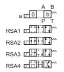
Type **TA**: 1 solenoid side A 2 external positions with return spring
