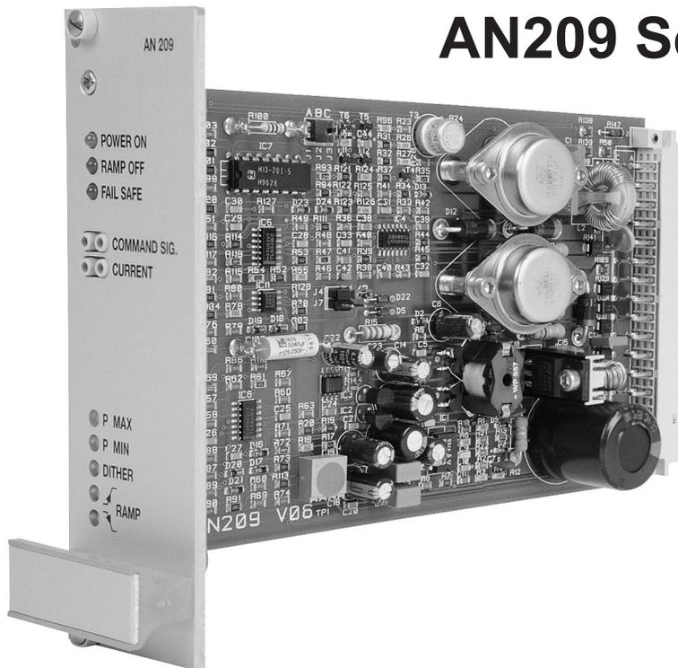
The AN209 servo amplifier has been designed to control single-magnet proportional valves and throttle-valves.
